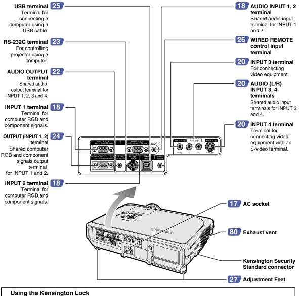
• This projector has a Kensington Security Standard connector for use with a Kensington MicroSaver Security System. Refer to the information that came with the system for instructions on how to use it to secure the projector.
